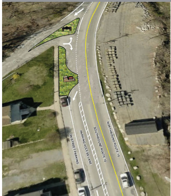
Existing conditions at Route 10 and Chapel Avenue (top) and potential traffic calming, aesthetic treatments and safety improvements (bottom)
