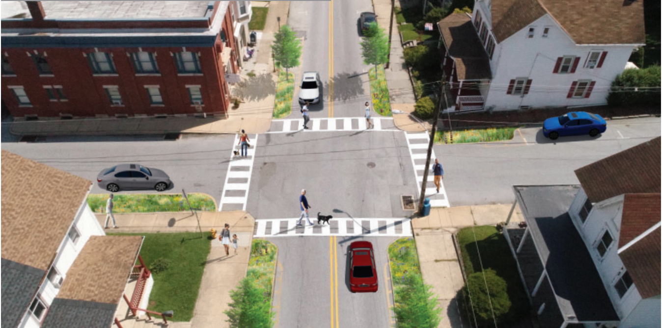
Raised planting beds can define the edges of an intersection slowing traffic, shortening crossing distance for pedestrians, and providing opportunities for stormwater management
